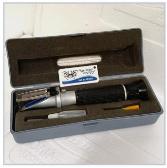
It is very important, for the measurement to be correct, that the liquid with which the calibration is performed and the refractometer itself have the same temperature (given the automatic temperature calibration range of this model between 10°C and 30°C, preferably below 20°C).
